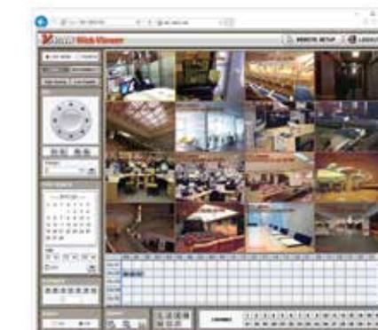
The VMAX A1™ has been designed to work with panoramic cameras like Digital Watchdog's STAR-LIGHT AHD PANO™ Panoramic camera. Each sensor is connected to the DVR as an individual output, resulting in a perfectly stitched panoramic view across the DVR's local monitor or the Pivot™ remote monitoring software.
