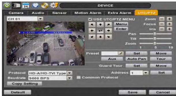
UTC is remotely set to camera OSD menu in the DVR. Select the proper protocol of the connected camera. Check the 'USE PTZ MENU' mode, set the menu and adjust as below.
