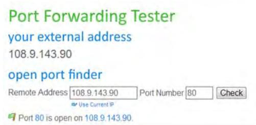
8. Once the router settings have been configured, open an internet explorer page and enter your router's external IP address:DVR's port number (for example: 72.243.193.215:81).
