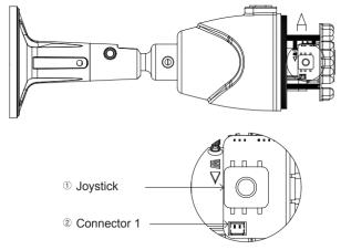
NOTE: Turn the front cover counter-clockwise and remove to access the OSD Contol Board.
