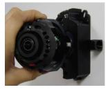
Adjust the camera lens position by using the 3-Axis Gimbal
