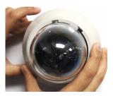
**6** Snap the dome cover over the camera module.
