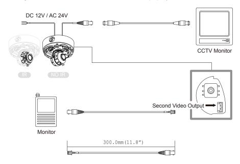
Power Connection: 12VDC & 24VDC Dual Voltage (Auto Polarity Detection and Protection) All cameras are equipped with a second video output for on-site configuration.
