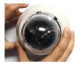
Adjust the camera lens, and snap the dome cover over the camera module
