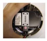
Squeeze the sides of the camera and separate the camera module from the dome cover.
