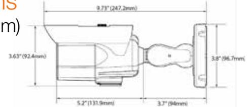
\* Dimensions based on the position of the sun shield cover
