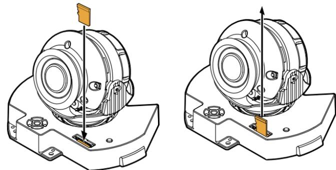
**NOTE:** Maximum SD Card size supported: 64GB. When inserting the SD card into the card slot, the SD card's contacts should be facing upward, as shown in the diagram.
