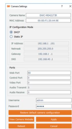
**i** 'Port forwarding' has to be set in your network's router for external access to the camera.
