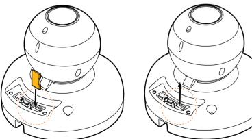
NOTE: Maximum SD Card size supported: 64GB. When inserting the SD card into the card slot, the SD card's contacts should be facing upward, as shown in the diagram.
