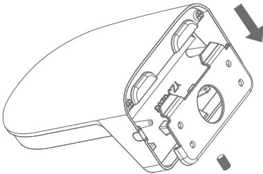
Separate the wall mount from the mounting template.
