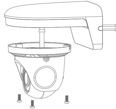
Attach the camera to the wall mount using the screws included with the camera.
