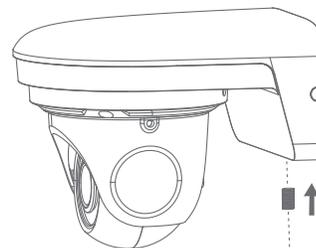
Connect the wall mount to the mounting bracket until secured. Use the small screw at the bottom of the wall mount to complete the installation.
