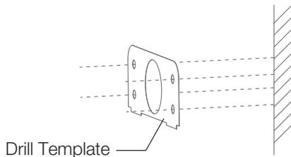
Use the mount's template to mark and drill the necessary holes in the wall.
