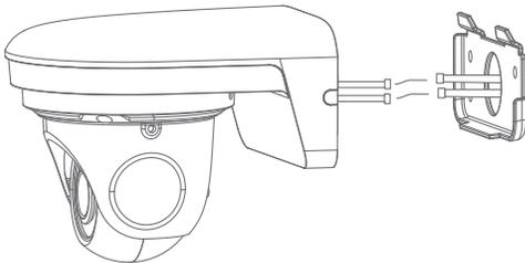
Pull wires through and make all necessary connections.
