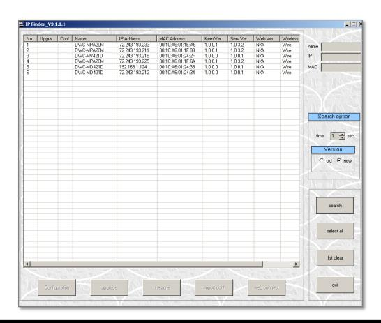
\*Make sure to install the IP Finder to a computer located on the same network segment (Subnet Mask) as the MEGAPIX camera.
