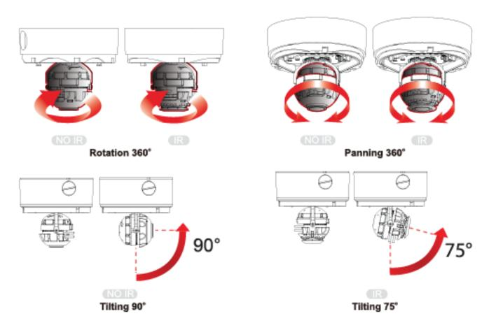
Do not over rotate the lens. Doing so will damage the camera lens module.
