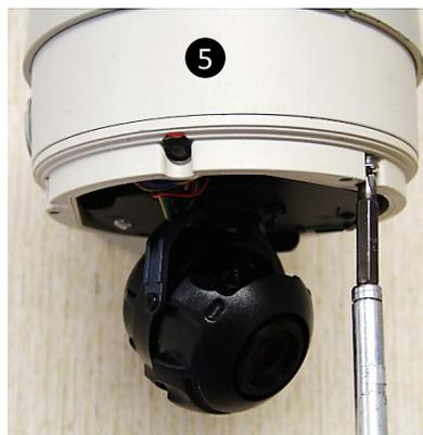
5. Connect all cables and snap the camera module onto the base.
