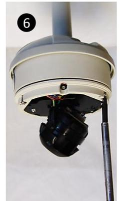
6. Attach the camera to the ceiling mount and secure the cover dome properly.
