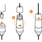
NOTE: To ensure moisture seal, make sure the o-ring is in place between and . In extreme environments use of an outdoor rated sealer is recommended.
