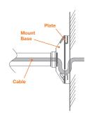
3. Cable passing through the wall with the junction box (Attention to the plate side)
