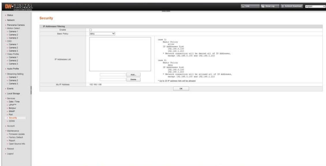
This menu allows you to restrict access to the camera according to IP addresses.
