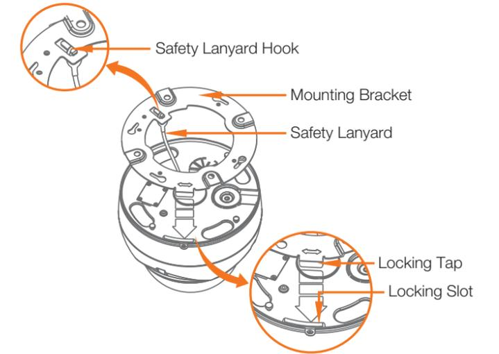
4. Mount and Twist the Dome to Fix.
