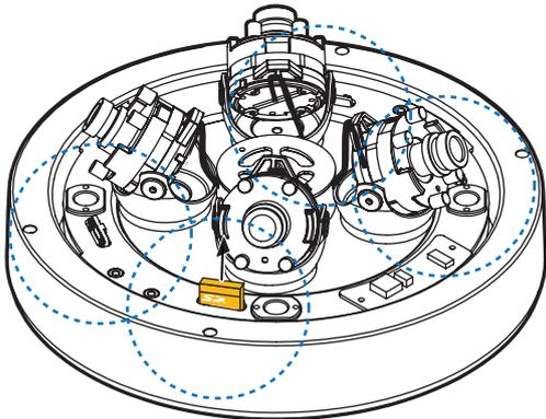
**2** Removing a SD Memory Card Gently press down on the exposed end of the memory card as shown in the diagram to eject the memory card from the slot.
