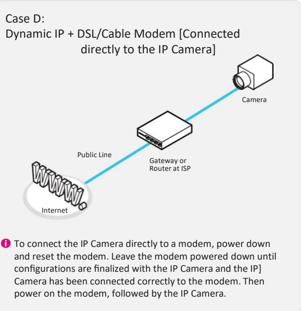
**i** To connect the IP Camera directly to a modem, power down and reset the modem. Leave the modem powered down until configurations are finalized with the IP Camera and the IP] Camera has been connected correctly to the modem. Then power on the modem, followed by the IP Camera.
