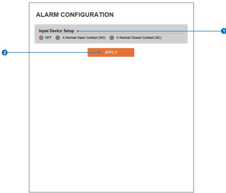
**1** **Input Device Setup** - Select input device type from OFF / N.O. / N.C.
