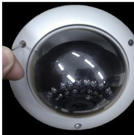
4. Attach the camera housing to the junction box using the assembly screws.
