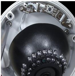
1. Pull wires through and make connections. Refer to page 10. Use mounting template to mount camera with dry wall mounts and wood screws.
