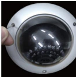
4. Secure the dome cover to the camera base by using the assembly screws. Make sure the camera is tightly secured to avoid damage to the camera module.
