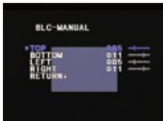
If MANUAL is selected, you can adjust the BLC levels in four areas of the scene (Top, Bottom, Left, Right). Increase the BLC levels to make the image brighter.
