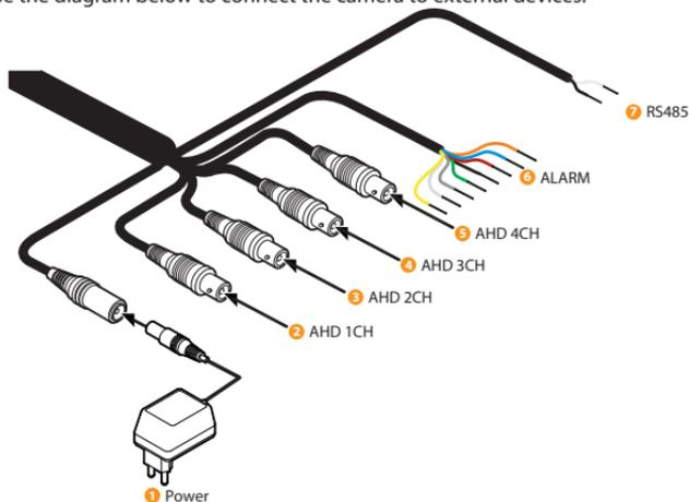
1. Power: connect the camera to a proper power supply. The camera supports both 12VDC and 24VAC. Below are the maximum power supplies for the camera:
