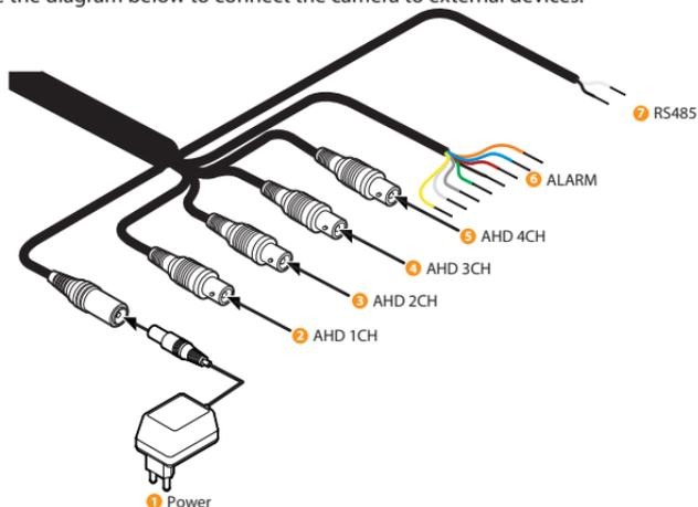
6. Alarm Input: Connect a sensor/alarm input device to the camera's alarm in+ and - cables.
