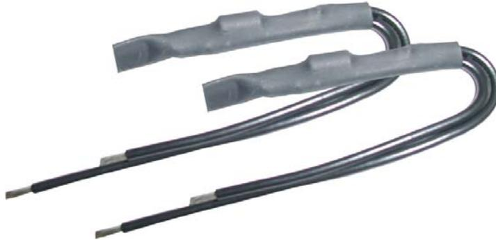
DITEK's DTK-ESS SPD (Surge Protective Device) protects electric door strikes. Electric door strikes (magnetic locks) are typically installed in metal frames, with low voltage wiring back to an access control panel, creating a vulnerable surge path. The compact ESS installs in the door frame to prevent voltage surges from getting into the control panel.
