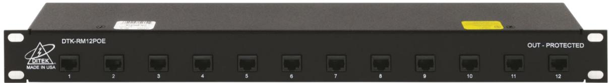
DITEK's DTK-RM12POE protects power, video and data circuits that use state-of-the-art Power over Ethernet connections. This 12-channel, 1U rack mount surge protector is compatible with CAT5e, CAT6 and CAT6A cabling infrastructure, and is ideal for installations where multiple Ethernet cabling feeds require protection before entering network switches.
