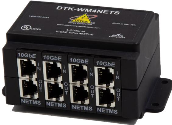
**DITEK's DTK-WM4NETS** is a 4-channel, wall mount surge protector that uses state-of-the-art circuitry to provide best-in-breed surge protection for shielded Ethernet, PoE and optional PoE extender\* circuits. It supports data speeds up to 10GbE, and provides surge protection grounding to remote devices when used with STP cabling. The DTK-WM4NETS is ideal for smaller installations where Ethernet cabling feeds require protection before entering network switches.
