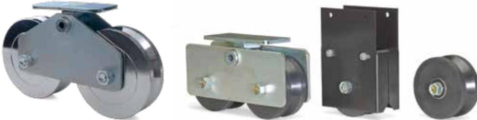
Available in sleeve and sealed roller bearings. Four inch and 6 inch sizes of either machined steel or UHMW. Maximum gate weights of up to 5000 lbs. V-Wheel assemblies include mounting bracket for 2x2 bottom rail. Tandem assemblies include pivoting mounting bracket. Tandem wheel assemblies provide superior performance for heavy gates by distributing the gate weight across 4 wheels instead of 2.
