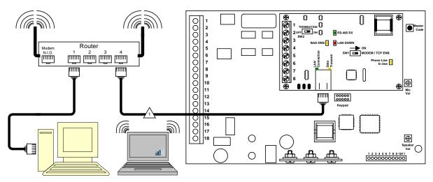
Wired or Wireless (if using a wireless router)
