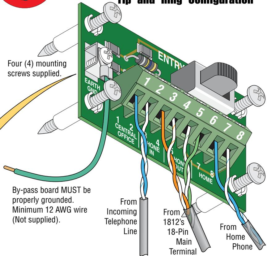
By-pass board **MUST** be properly grounded. Minimum 12 AWG wire (Not supplied).
