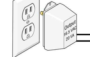
The 1812 Plus operates **ONLY** on 16.5 VAC. **DO NOT** power the 1812 with 24 Volt transformer or source voltage. Use the supplied power transformer, 16.5 VAC, 20 VA (or UL listed equivalent) to power the telephone entry system. **DO NOT** power any other devices (electric strikes, magnetic locks, additional 1812s etc.) from the 1812's power transformer. **See previous page for wire size and run distances.**
