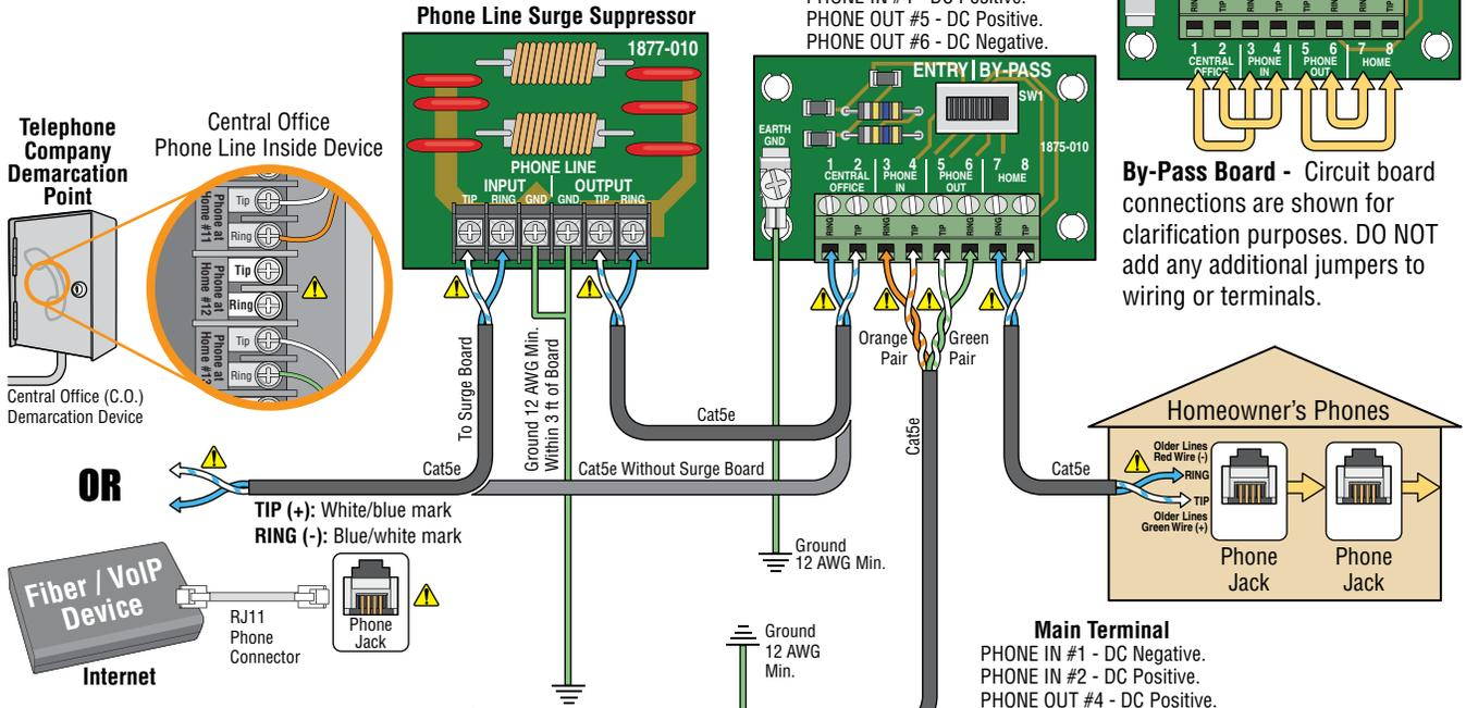
**Main Terminal** - Circuit board connections are shown for clarification purposes. **DO NOT** add any additional jumpers to wiring or terminals.
