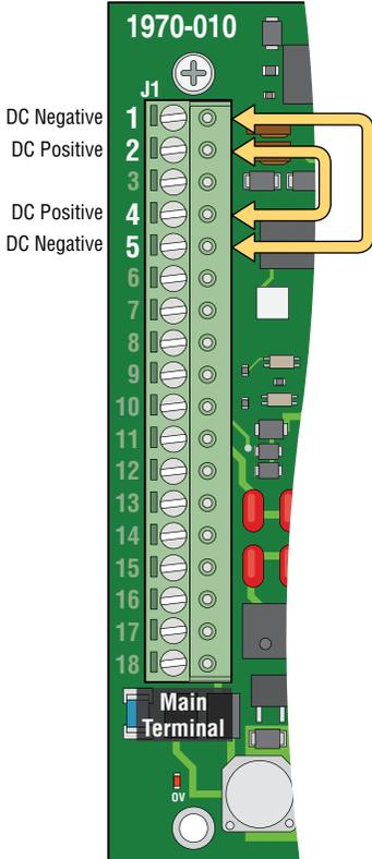
Check that all boards are **properly grounded** with 12 AWG gauge wire minimum.
