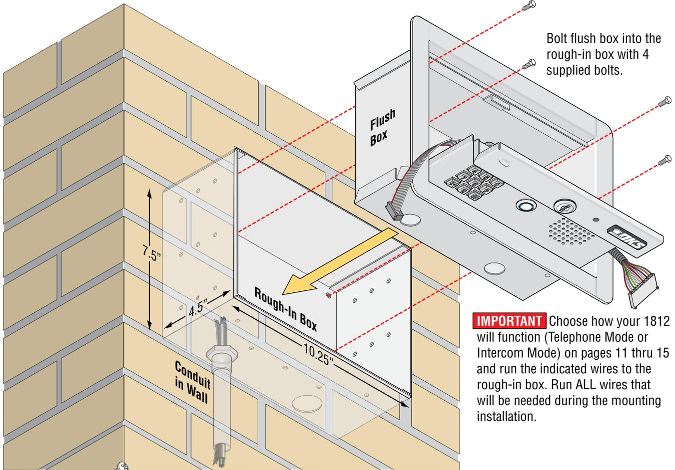
Bolt flush box into the rough-in box with 4 supplied bolts.
