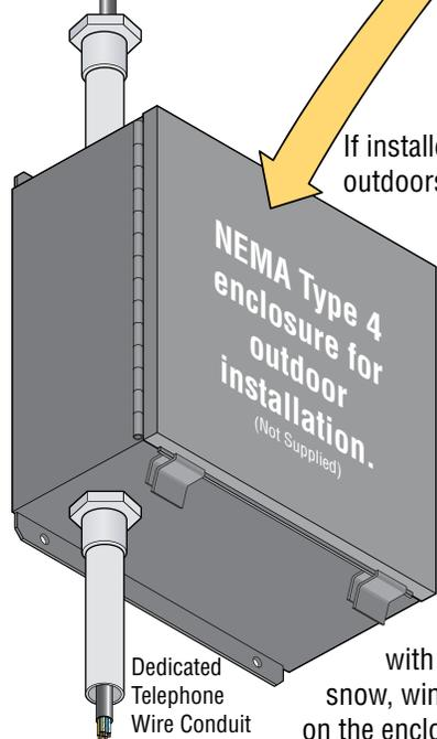
Use only twisted pair telephone wire that is rated for direct underground burial. **DO NOT** use wire that is intended for indoor applications. **Recommend Cat5e Gel Filled (flooded) UV Resistant Direct Burial Cable in conduit.** **DO NOT** run telephone wires and high voltage wires in the same conduit. It is recommended to run all necessary wires to the by-pass board in a “dedicated” telephone wire conduit. Check the phone wire chart on next page for wire size and distances.
