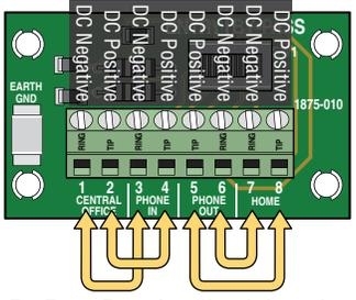
**By-Pass Board** - Circuit board connections are shown for clarification purposes. **DO NOT** add any additional jumpers to wiring or terminals.
