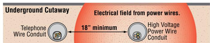
**Note:** Do not run telephone wires and high voltage power wires in the same conduit. Separate the high voltage conduit and the telephone conduit by at least 18 inches to prevent any electrical field interference that could occur.
