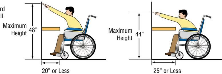
**3. Unobstructed Side Reach.** Where a clear floor or ground space allows a parallel approach to an object and the side reach is **unobstructed**, and the edge of the clear floor space is **10 inches** (255 mm) maximum from the object, mounting height shall be a minimum of **15 inches** (380 mm), and a maximum of **48 inches** (1.22 m), above the floor or ground to the operable controls.
