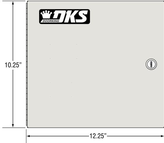
**WARNING!** If this entry system is used to control a vehicular gate with an automatic gate operator, the entry system must be mounted a minimum of six (6) feet away from the gate and gate operator, or in such a way that a person cannot operate the entry system and touch the gate or gate operator at the same time.
