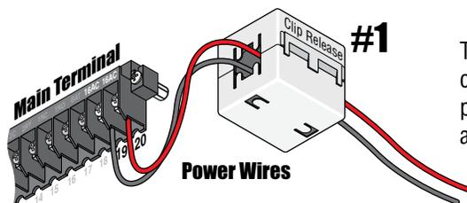
To install the ferrite filter, release the clip on the side to open the filter, place the wires in the circular core and snap the filter closed.
