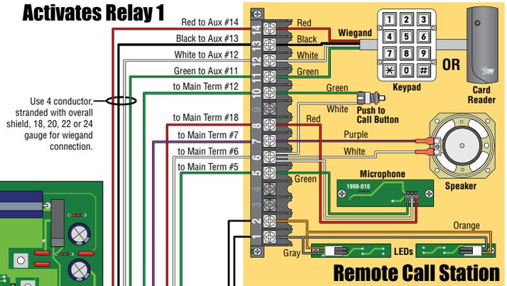
**#5 & #6 - 16.5 VAC Output:** Can be used to power remote call station. Power wire polarity does not matter.
