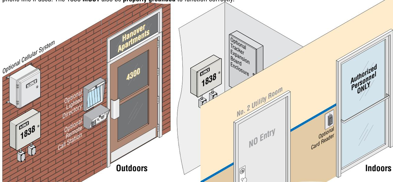
**WARNING** If this multi-door access controller is used to control a vehicular gate with an automatic gate operator, the access controller must be mounted a minimum of six (6) feet away from the gate and gate operator, or in such a way that the user cannot come into contact with the gate or gate operator when using this access controller .
