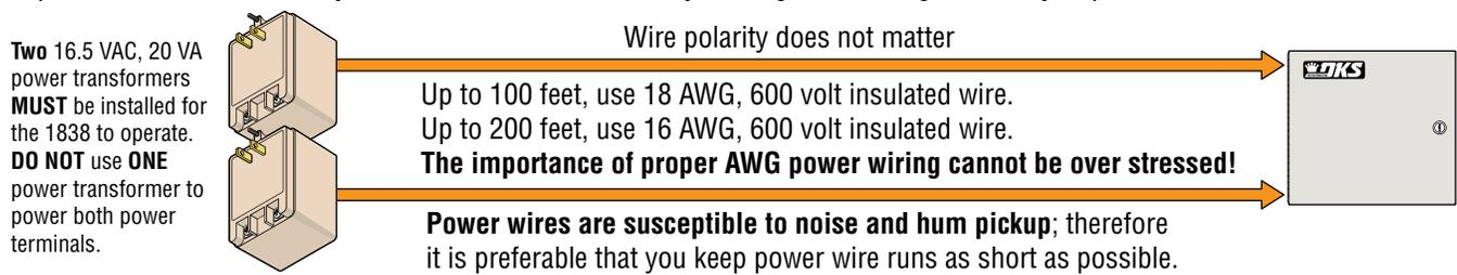
**Do Not Connect To A Receptacle Controlled By A Switch.**
