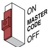
The master code switch **MUST** be kept in the **OFF** position for normal operation. Turn the master code switch **ON** only when programming the system's master code. See section 3.2.1 to program the system's master code. If the master code switch is **turned ON** and a new master code is **NOT** entered, the system will sound a long tone after approximately 30 seconds. This tone will continue every 30 seconds until a new master code is entered, or until the switch is turned off.
