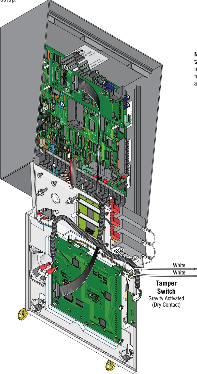
**Note:** To comply with UL 294 Standard for Safety, the tamper switch provided in this access control equipment must be set to activate an alarm or alarm signal when tripped. If the tamper switch is **NOT** connected to activate an alarm or alarm signal, **this will void UL 294 certification.**
