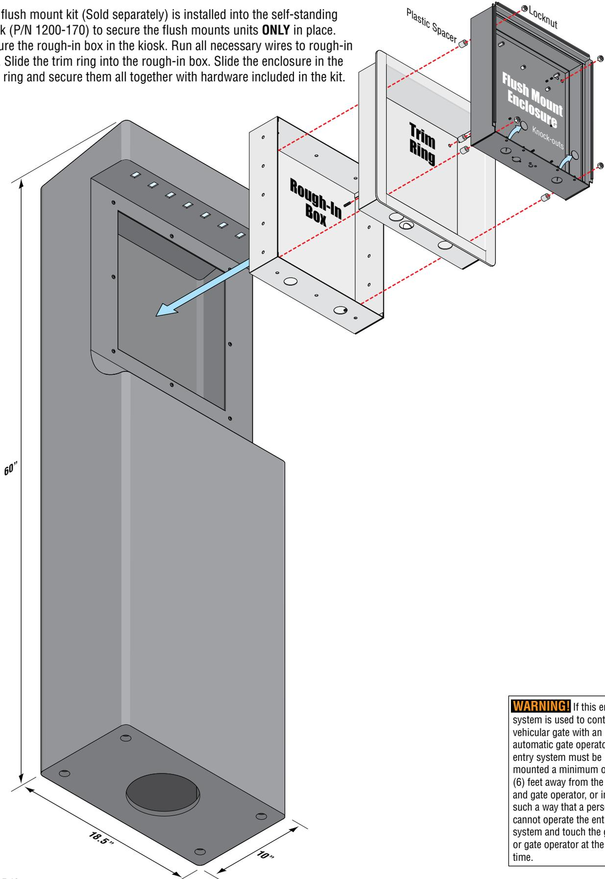
**WARNING!** If this entry system is used to control a vehicular gate with an automatic gate operator, the entry system must be mounted a minimum of six (6) feet away from the gate and gate operator, or in such a way that a person cannot operate the entry system and touch the gate or gate operator at the same time.
