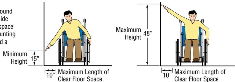
**4. OBSTRUCTED HIGH Side Reach.** If the side reach is over an obstruction **10 inches or less**, mounting height shall be a maximum of **48 inches** (1.21 m) above the floor or ground to the operable controls. If the side reach is over an obstruction **greater than 10 inches, but less than 24 inches**, mounting height shall be a maximum of **46 inches** (1.17 m) above the floor or ground to the operable controls.
