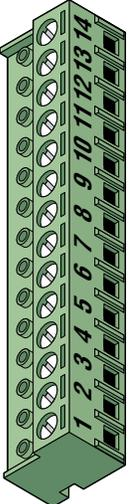
**Note:** The 14-pin aux terminal can be removed for easy wiring. Expansion boards are connected here when used.
