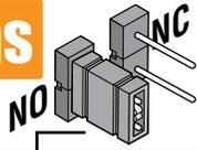
**Relay 2 Note:** Normally Open and Normally Closed relay jumper is used to set **Relay 2** input on the circuit board (See section 4.6).
