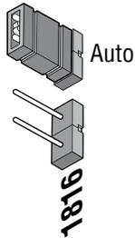
This jumper sets the system to operate as a **stand-alone unit - AUTO** (top position), or to interface with the 1816 Telephone Intercom System (bottom position). The jumper is set to **AUTO from the factory**.
