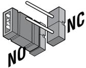
This jumper sets the contacts on relay number two at either Normally Open (NO) or Normally Closed (NC). The jumper is set to **NO from the factory**.
