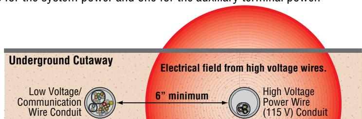
**Wiegand wire runs are 500-foot maximum.** Use 6-conductor stranded wire with overall shield. 18, 20, 22 or 24 gauge is sufficient for these connections.
