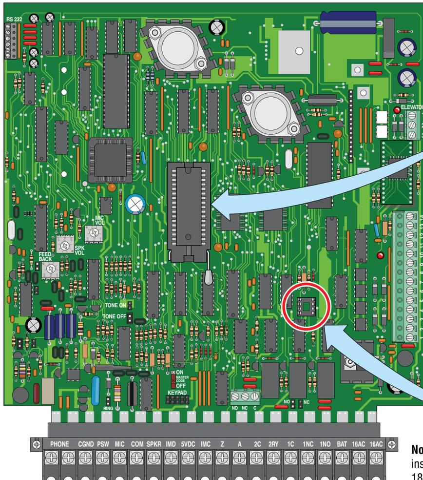
**Dimple MUST be at the top of the chip!**
