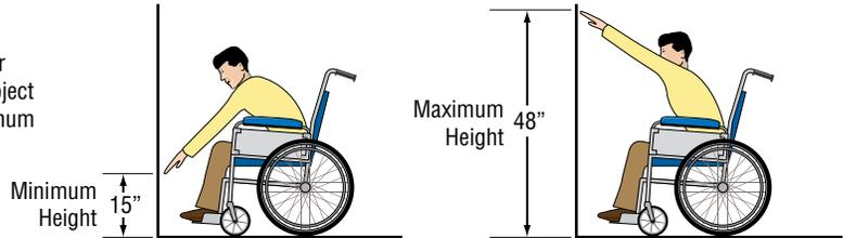
**2. OBSTRUCTED HIGH Forward Reach.** If the high forward reach is over an obstruction, reach and clearances shall be as shown. **NOTE: If the height of a control is 48" maximum, then the length of the obstruction must be 20" or less. If the height of a control is 44" maximum, then the length of the obstruction may be increased to 25" or less.**
