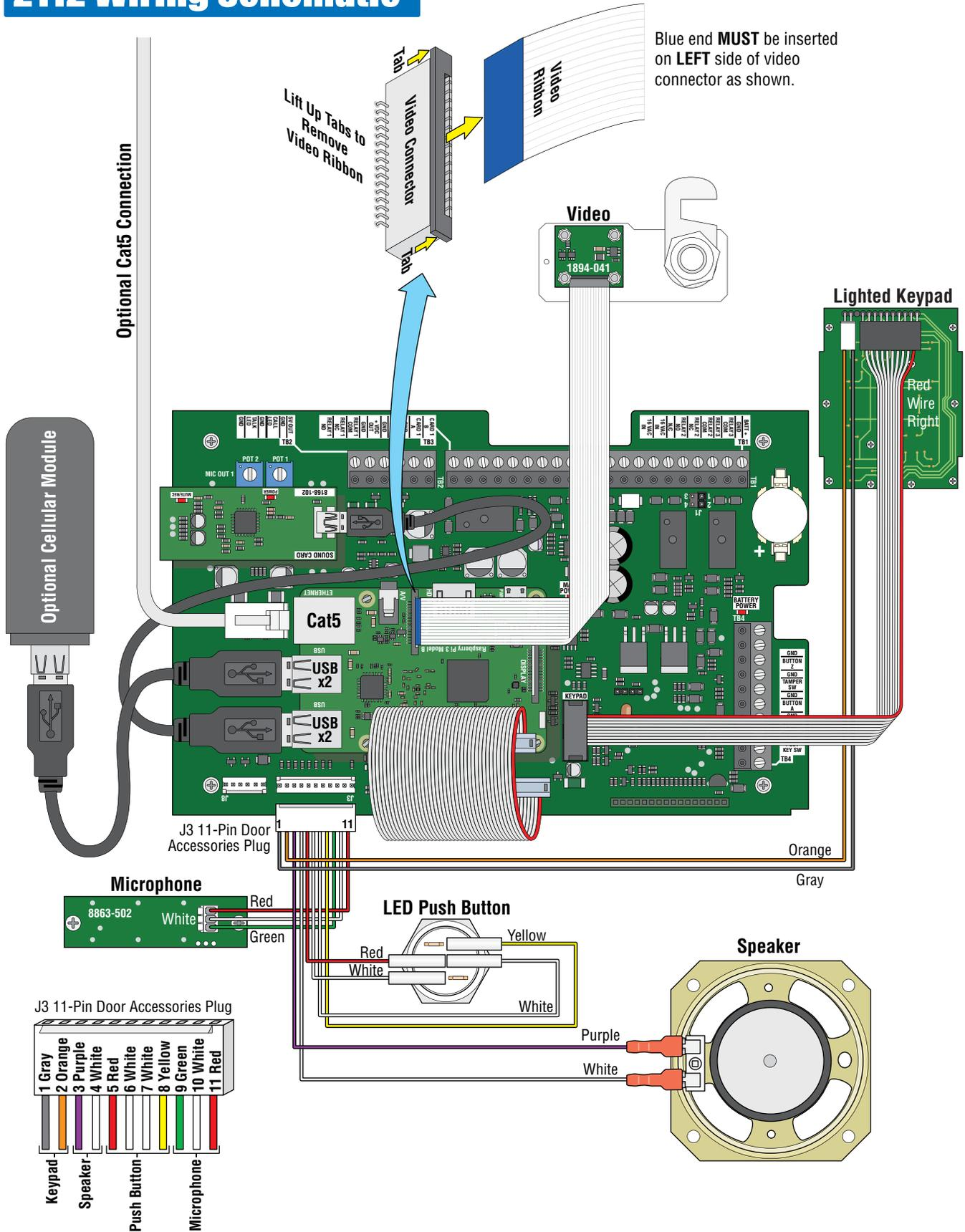
Blue end **MUST** be inserted on **LEFT** side of video connector as shown.
