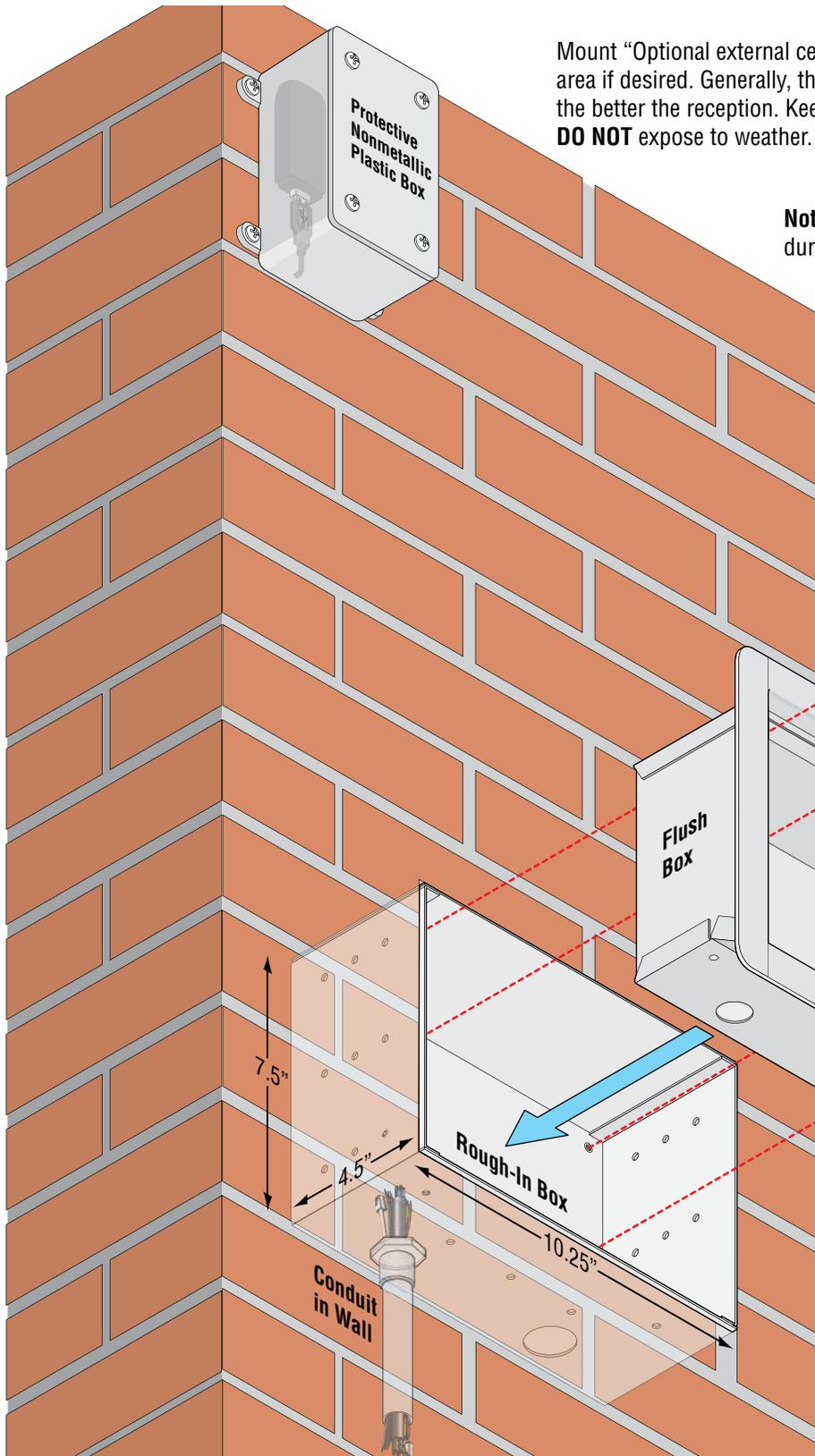
Mount "Optional external cellular module kit" in a **secure protected** area if desired. Generally, the higher the cellular module is mounted, the better the reception. Keep clear of metal. **DO NOT** expose to weather.
