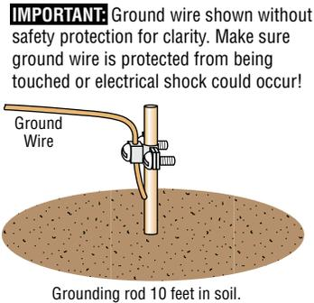
**IMPORTANT:** Ground wire shown without safety protection for clarity. Make sure ground wire is protected from being touched or electrical shock could occur!
