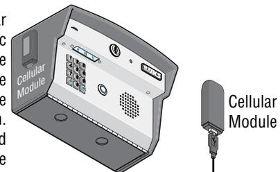
**Flush Mount:** Cellular module needs to be mounted **outside** metal enclosure in a **protected secure** area as high as possible for best reception. Avoid **any** metal around module. **DO NOT** expose module to weather. See pages 7 & 8.
