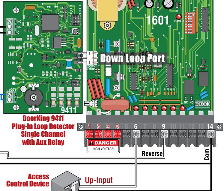
**Typical DIP-Switch settings when using a 9411 Loop Detector with a Down Loop and a Access Control Device**
