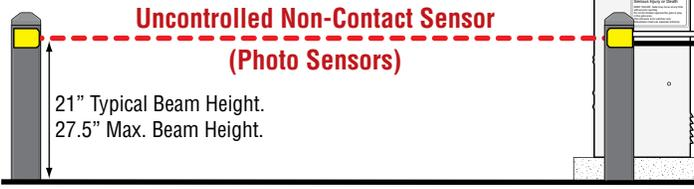
**Uncontrolled Non-Contact Sensors Note:** Helps minimize the potential of the arm lowering on vehicular or other traffic that loops cannot sense. **Lowering arm will always reverse when beam gets blocked.** See next page for CONTROLLED non-contact sensor layout.
