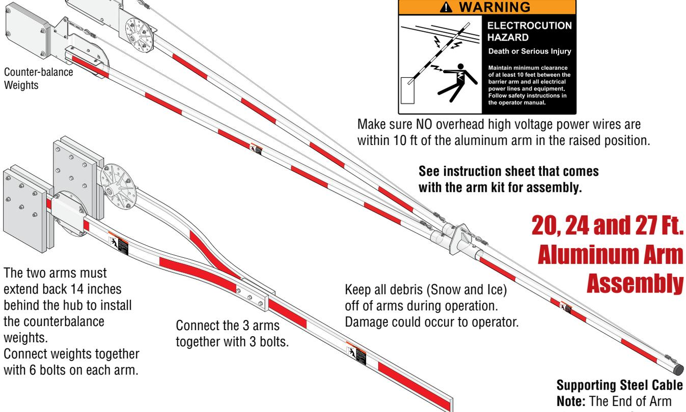
The two arms must extend back 14 inches behind the hub to install the counterbalance weights. Connect weights together with 6 bolts on each arm.
