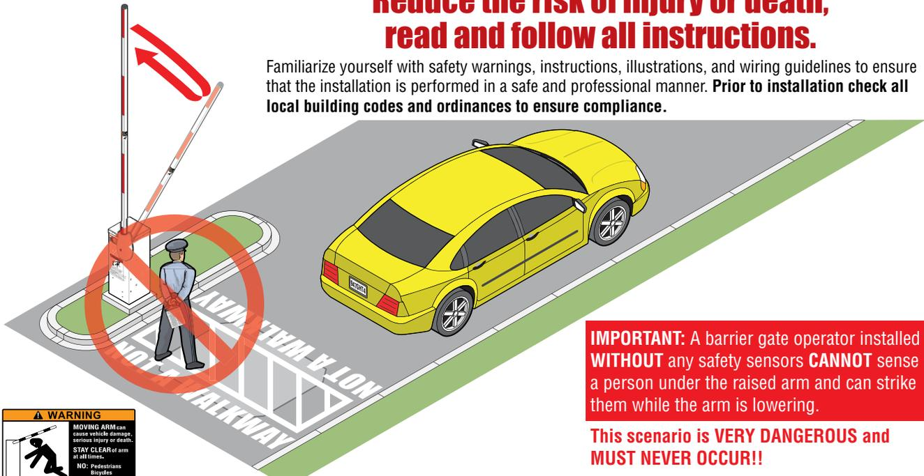
**IMPORTANT:** A barrier gate operator installed **WITHOUT** any safety sensors **CANNOT** sense a person under the raised arm and can strike them while the arm is lowering.
