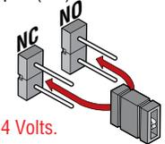
Contact rating is 1 amp maximum at 24 Volts.
