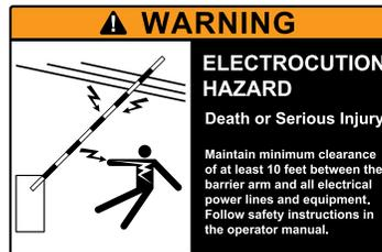
Make sure **NO** overhead high voltage power wires are within 10 ft of the aluminum arm in the raised position.
