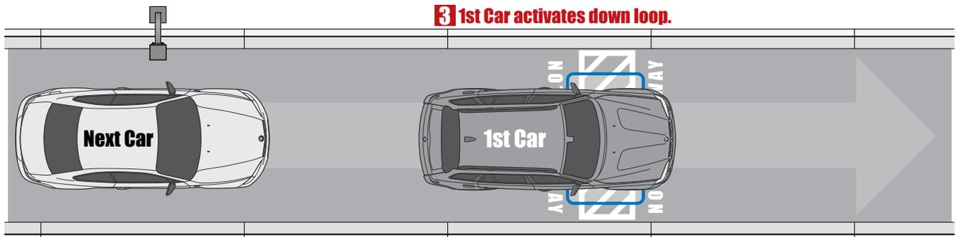
**4 While 1st Car is on down loop, the next UP command is given.**
