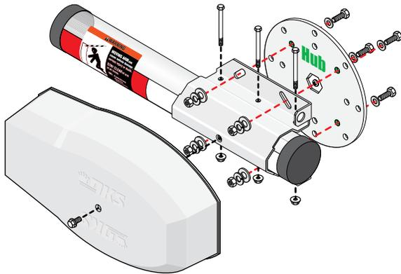
**Lighted Arm Note:** Unplug wire harness and remove from operator housing **BEFORE** unbolting arm from hub.
