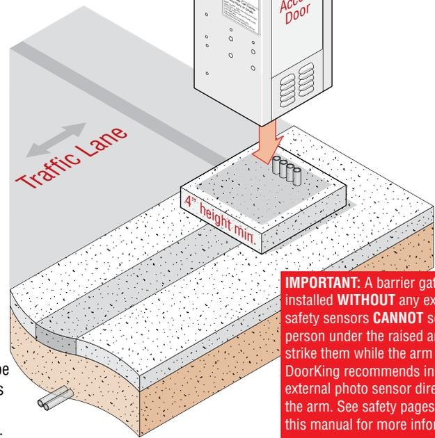
**IMPORTANT:** A barrier gate operator installed **WITHOUT** any external safety sensors **CANNOT** sense a person under the raised arm and can strike them while the arm is lowering. DoorKing recommends installing an external photo sensor directly under the arm. See safety pages in front of this manual for more information.
