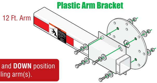
Test hub **UP** and **DOWN** position before installing arm(s).
