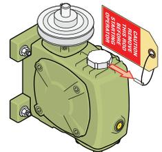
Remove breather pin from gear reducer **AFTER** the operator has been secured in place.
