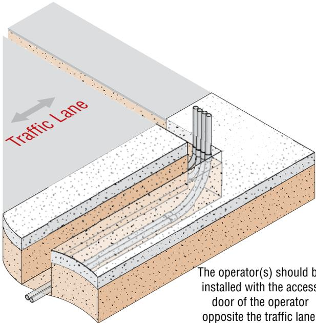
The operator(s) should be installed with the access door of the operator opposite the traffic lane.
