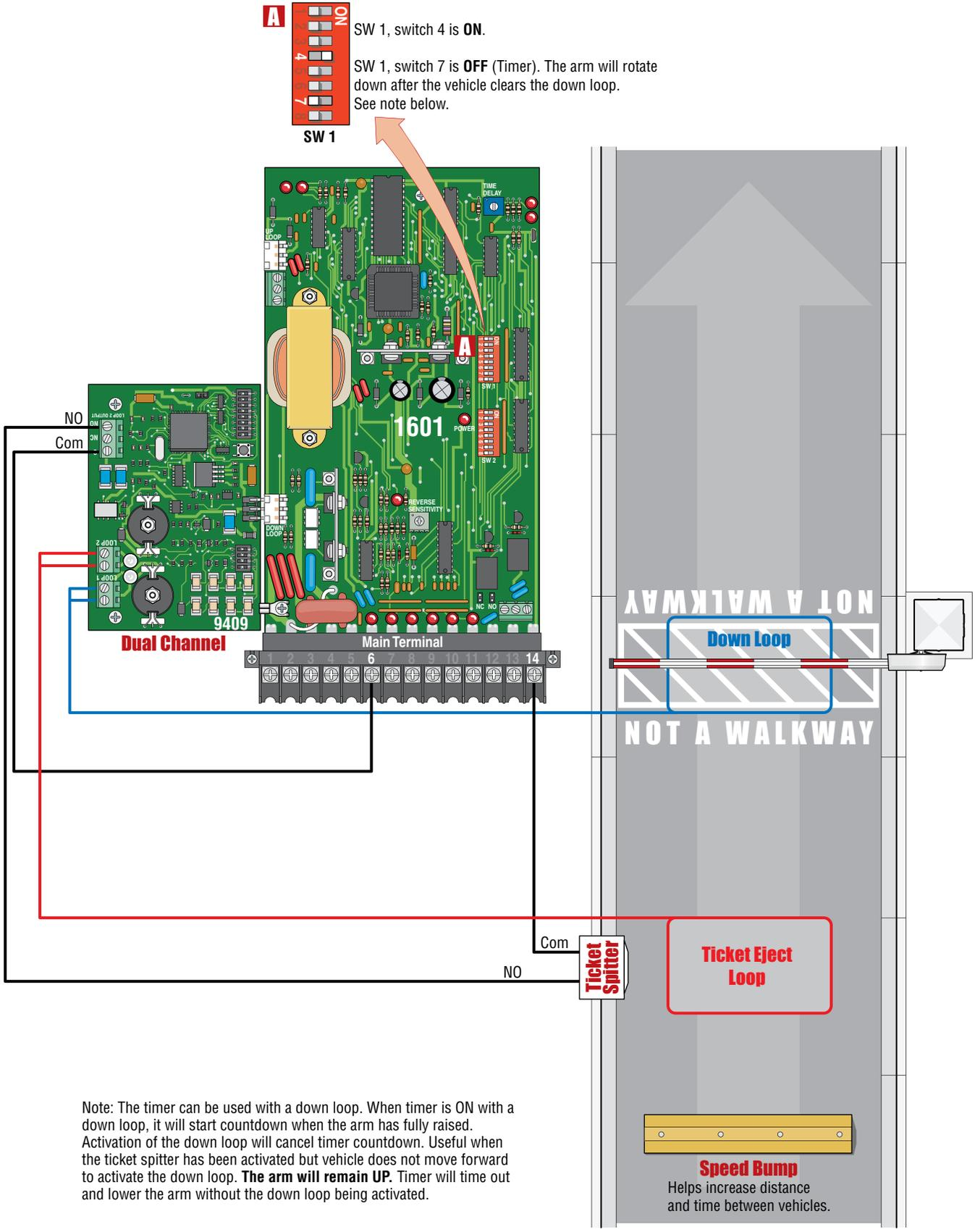
Note: The timer can be used with a down loop. When timer is ON with a down loop, it will start countdown when the arm has fully raised. Activation of the down loop will cancel timer countdown. Useful when the ticket spitter has been activated but vehicle does not move forward to activate the down loop. **The arm will remain UP.** Timer will time out and lower the arm without the down loop being activated.
