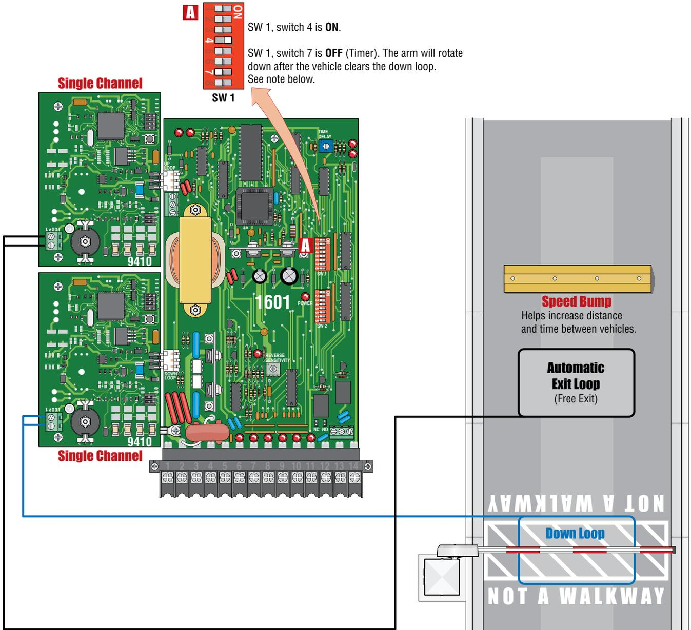
Note: The timer can be used with a down loop. When timer is ON with a down loop, it will start countdown when the arm has fully raised. Activation of the down loop will cancel timer countdown. Useful when the automatic exit loop has been activated but vehicle does not move forward to activate the down loop. **The arm will remain UP.** Timer will time out and lower the arm without the down loop being activated.
