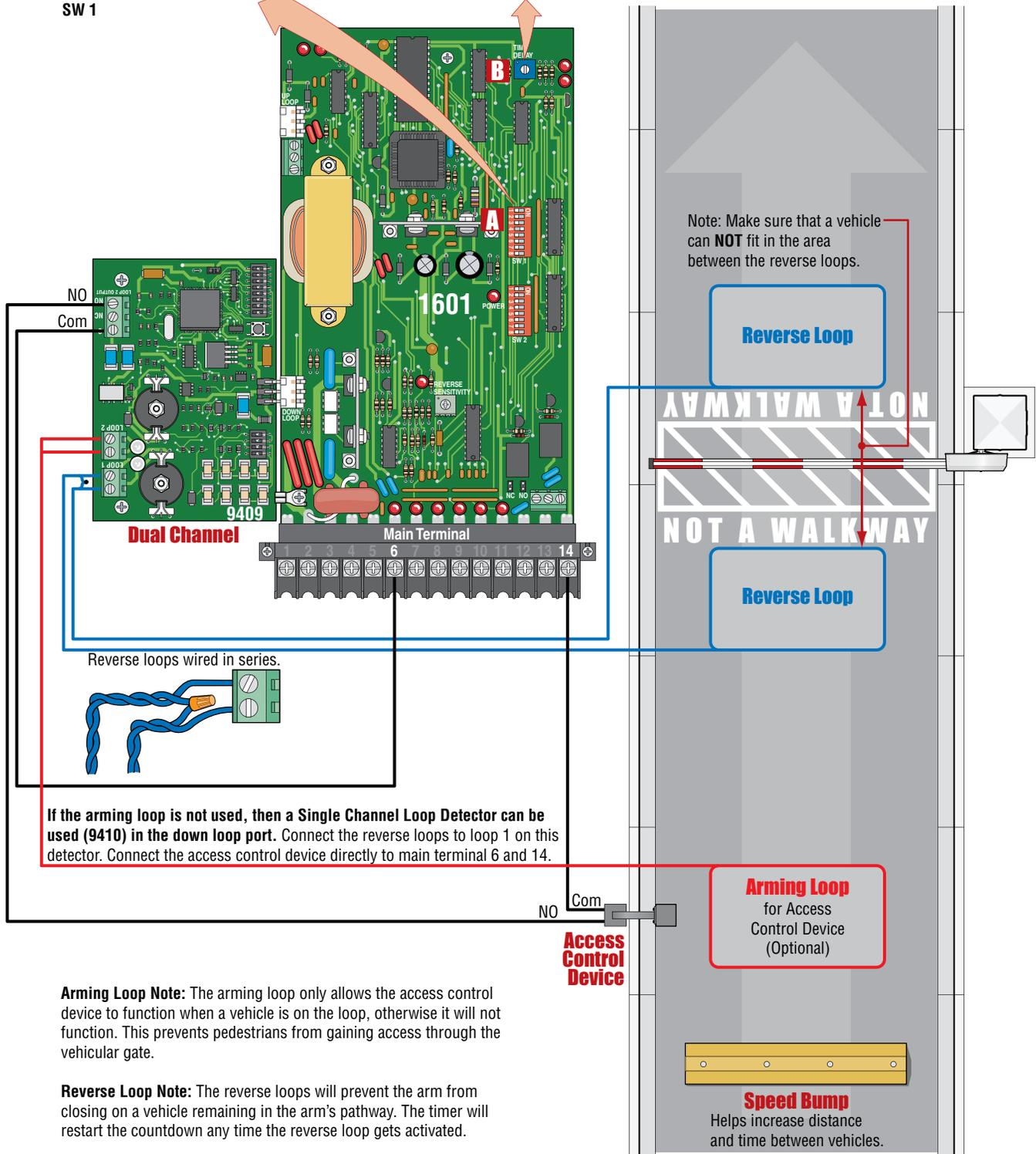
If the arming loop is not used, then a Single Channel Loop Detector can be used (9410) in the down loop port. Connect the reverse loops to loop 1 on this detector. Connect the access control device directly to main terminal 6 and 14.
