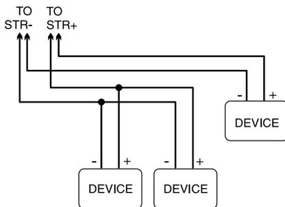
The wiring length of each addressable loop is restricted to the following distances, depending on the amount of current required (see Section 2.2 “Calculating Current Draw”). Consult the wiring chart on the next page.
