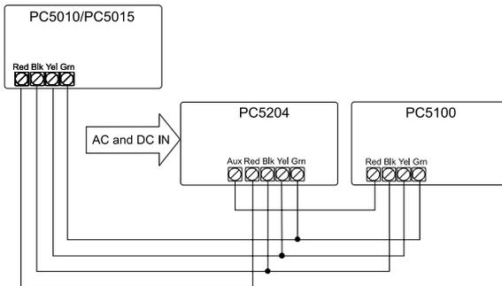
After wiring is complete, add power back to the PC5010/PC5015. The system will detect the new module and it will be supervised.
