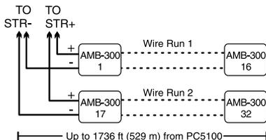
**!** *Not more than four 24AWG conductors should be connected to a single terminal as wire bulk may cause improper operation.*
