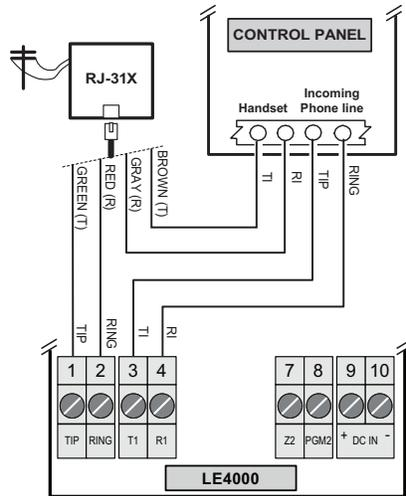
Figure 8-2 Telephone connection
