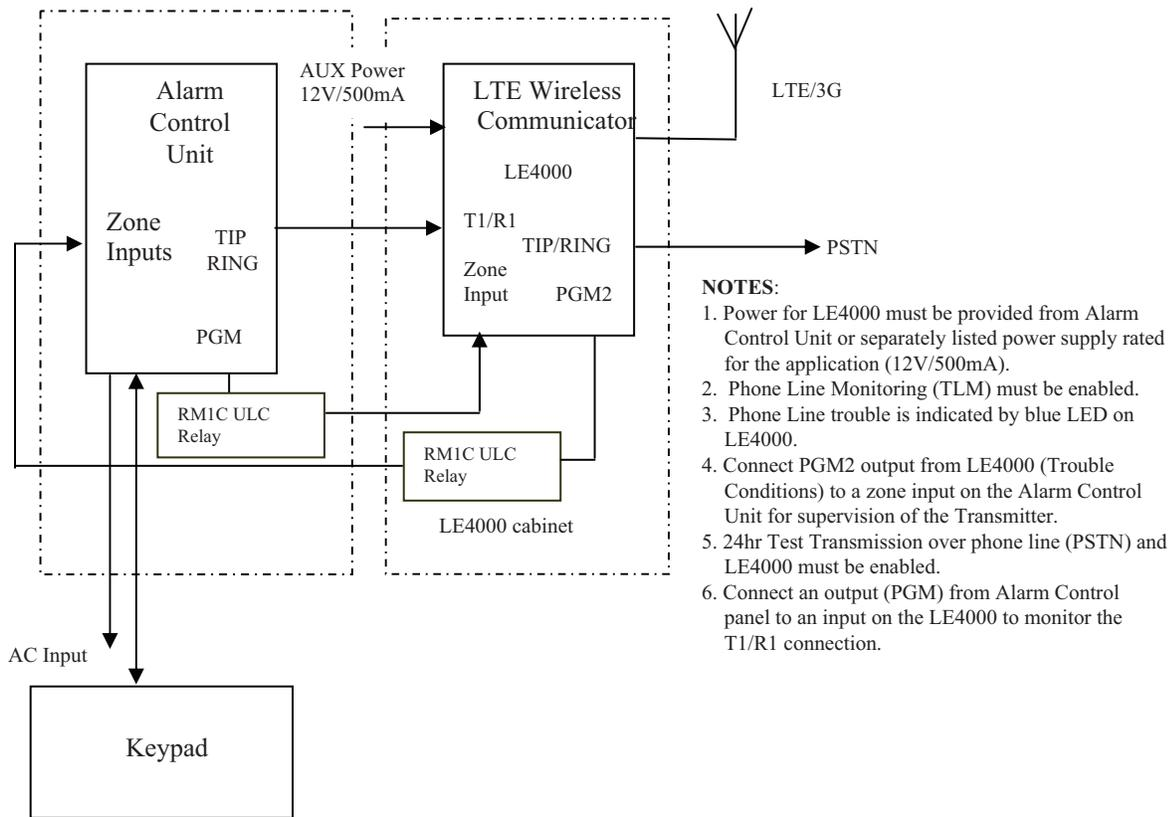
Figure 8-4 Alarm control unit and LTE/3G transmitter
