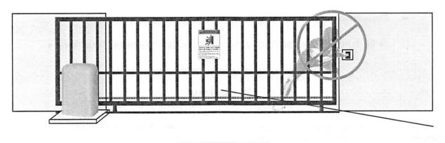
Regarding Ornamental Grill Styled Gates: Injuries may be avoided if a mesh or screen is installed on the gate. Injuries resulting from hands and feet becoming stuck in gate or children riding the gate while in movement, can be greatly reduced if this "screen" or "mesh" is applied to gate as a safety precaution.
