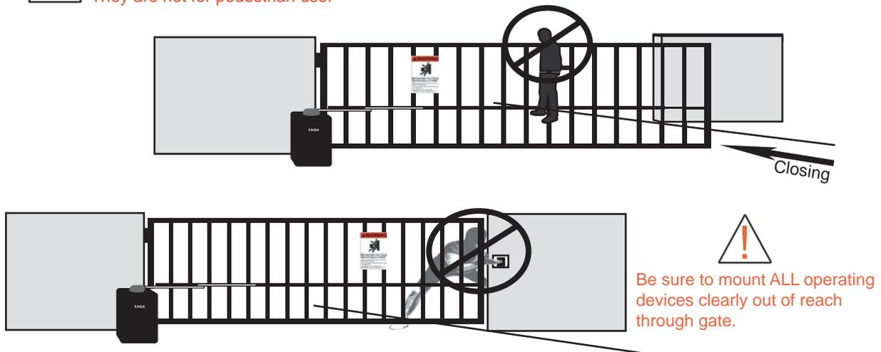
Regarding Ornamental Grill Styled Gates: Injuries may be avoided if a mesh or screen is installed on the gate. Injuries resulting from hands and feet becoming stuck in gate or children riding the gate while in movement, can be greatly reduced if this "screen" or "mesh" is applied to gate as a safety precaution.
