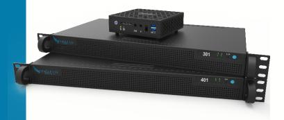
The Eagle Eye Bridge models receive and analyze video streams, provide on-premise buffering for bandwidth management, detect any camera issues and automatically transmit camera and system status information to the Eagle Eye Cloud Data Center. The Eagle Eye Bridge models support up to 30 HD IP cameras.
