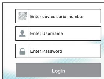
**Device Serial Number:** Click
