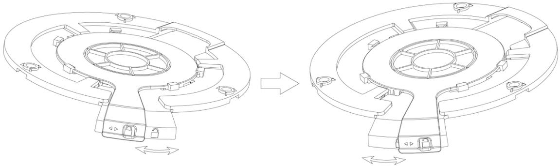
**Step 4** Pull the device cable out through mounting surface or the cable tray on the bottom of the device.
