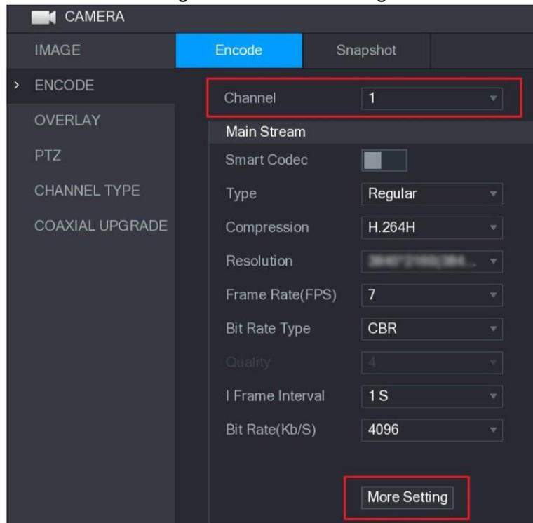
**Step 2** In the **Channel** list, select the camera that you want to configure according to the coaxial port number.
