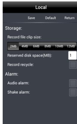
**Storage:** Set the relevant parameters of mobile video. Only when the SD card is inserted do the storage settings take effect.
