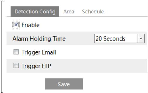
1. Enable line crossing alarm and set the alarm holding time.
