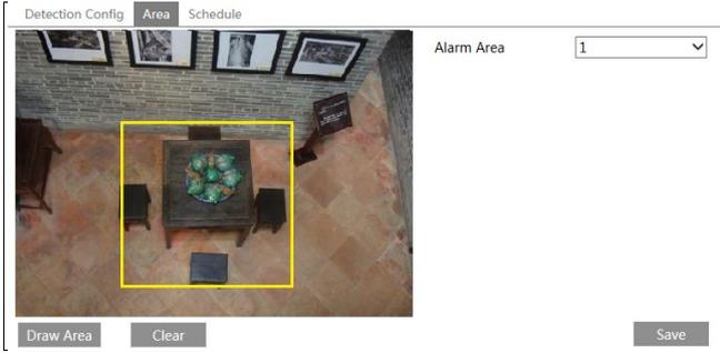
Set the alarm area number on the right side. Only one alarm area can be added. Click the “Draw Area” button and then click around the area where you want to set as the alarm area in the image on the left side (the alarm area should be a closed area). Click the “Stop Draw” button to stop drawing. Click the “Clear” button to delete the alarm area. Click the “Save” button to save the settings.
