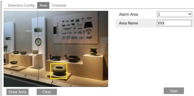
Set the alarm area number and then enter the desired alarm area name. Only one alarm area can be added. Click the “Draw Area” button and then click around the area where you want to set as the alarm area in the image (the alarm area should be a closed area). Click the “Stop Draw” button to stop drawing. Click the “Clear” button to delete the alarm area. Click the “Save” button to save the settings.
