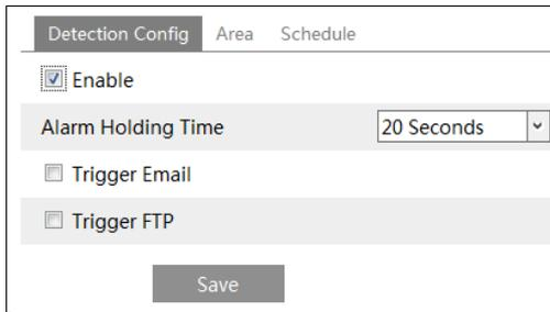
1. Enable region intrusion detection alarm and set the alarm holding time.
