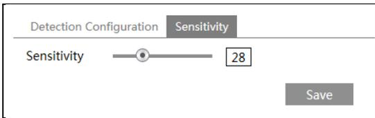
Drag the slider to set the sensitivity value or directly enter the sensitivity value in the textbox. Click “Save” button to save the settings.
