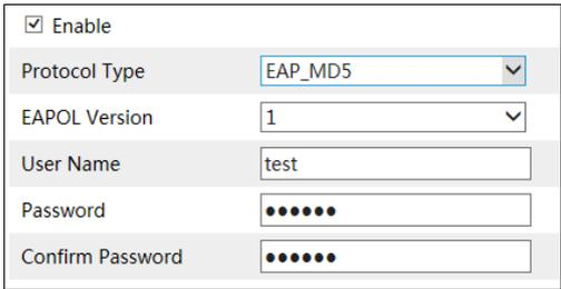
To use this function, the camera shall be connected to a switch supporting 802.1x protocol. The switch can be reckoned as an authentication system to identify the device in a local network. If the camera connected to the network interface of the switch has passed the authentication of the switch, it can be accessed via the local network.
