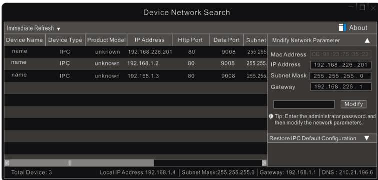
③ Modify the IP address. The default IP address of this camera is 192.168.226.201. Click the information of the camera listed in the above table to show the network information on the right hand. Modify the IP address and gateway of the camera and make sure its network address is in the same local network segment as the computer's. Please modify the IP address of your device according to the practical situation.
