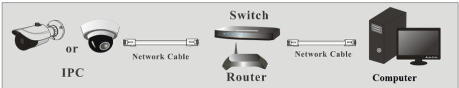
① Make sure the PC and IP-Cam are connected to the local network and the IP-Tool is installed in the PC from the CD.
