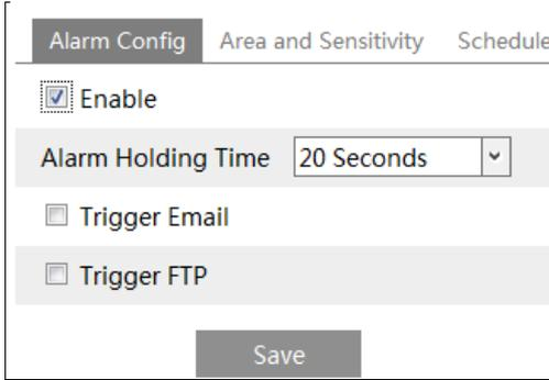
1. Check “Enable” check box to activate motion based alarms. If unchecked, the camera will not send out any signals to trigger motion-based recording to the NVR or CMS, even if there is motion in the video.
