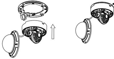
⑤ Three-axis adjustment. Before adjustment, preview the image of the camera on a monitor and then adjust the camera according to the figure below to get an optimum angle.
