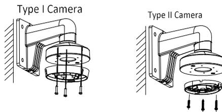
Figure 2-18 Install the Mounting Base to the Bracket
