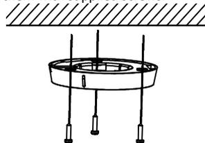
Figure 2-3 Attach the Mounting Base to the Ceiling
