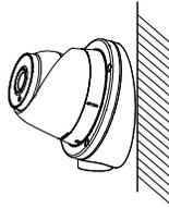
Figure 2-9 Fix the Camera to the Inclined Base
