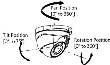
Figure 2-14 3-axis Adjustment
