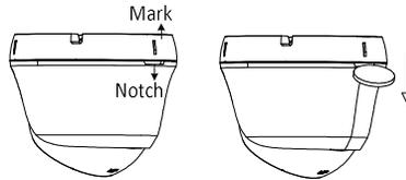
Figure 2-1 Disassemble the Camera
