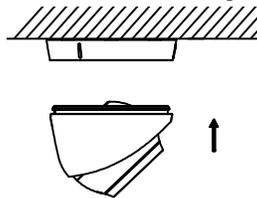
Figure 2-4 Secure the Camera with Mounting Base
