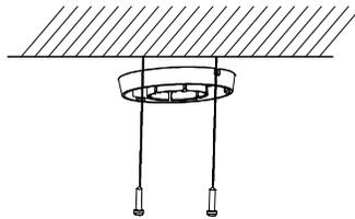
Figure 2-21 Attach the Mounting Base to the Ceiling
