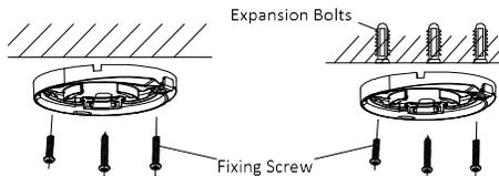
Figure 2-12 Fix the Mounting Base to the Ceiling
