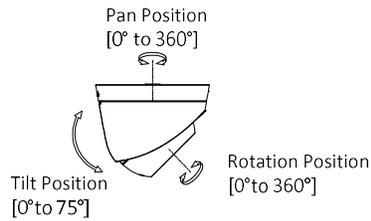
Figure 2-23 3-axis Adjustment
