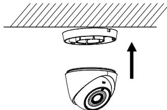
Figure 2-22 Secure the Camera with Mounting Base
