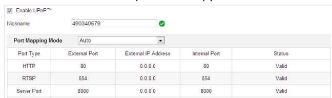
The screenshot shows the UPnP settings interface. At the top, there is a checkbox labeled "Enable UPnP™" which is checked. Below it is a "Nickname" field with the value "490340679" and a green checkmark. Underneath is a "Port Mapping Mode" dropdown menu set to "Auto". Below the dropdown is a table with the following data:
