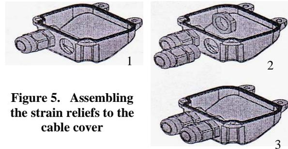
**Figure 5. Assembling the strain reliefs to the cable cover**
