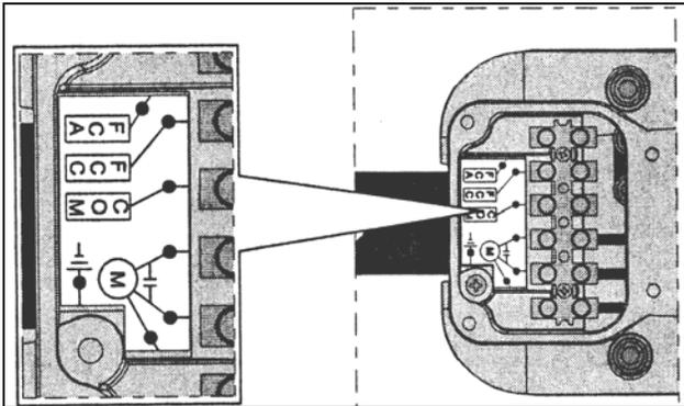
**Figure 3. Electric Cable Detail Sticker**
