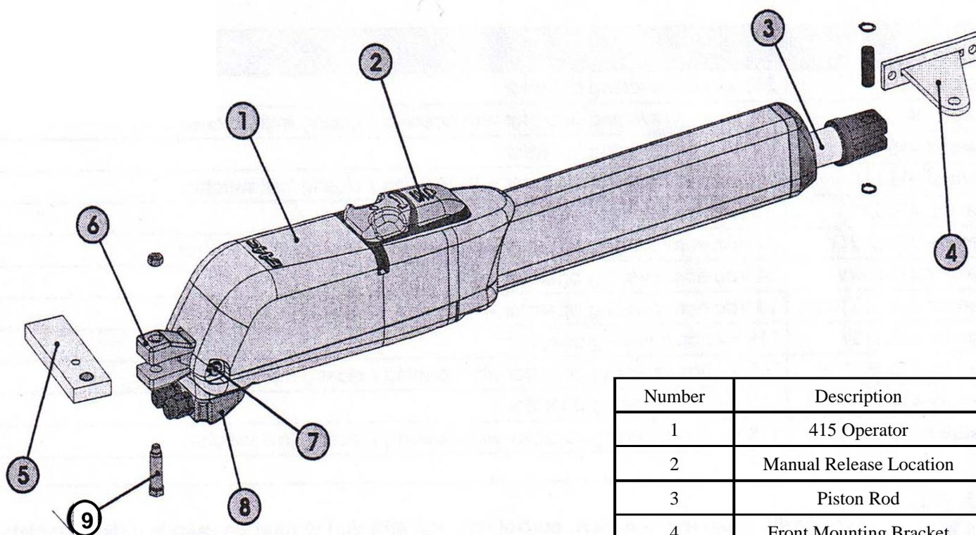
Figure 1. Parts of the 415 L LS Operator
