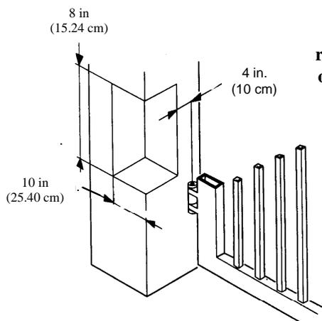
**Figure 7. The required dimensions of the recessed liner when notching the gate post**
