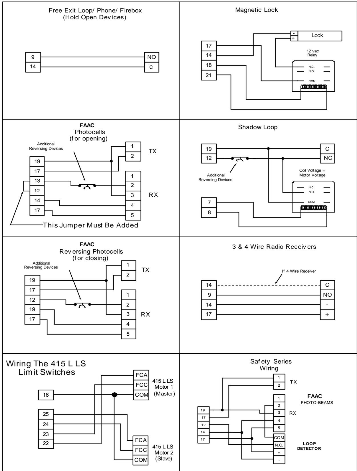
NO = Normally Open, NC = Normally Closed, C = Common, TX = Transmitter, RX = Receiver
