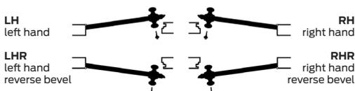
The hand is determined by the direction the door swings when viewed from the exterior or corridor side of the door.
