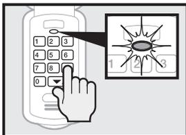
The Keypad's LED will flash on and off each time you press a key indicating the keypad has accepted each entry.
