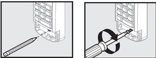
5. Mark and drill a pilot hole for the bottom screw and secure keypad to wall (**DO NOT** overtighten).
