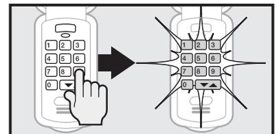
The Keypad's LED and Program key will light. Keypad will flash quickly if you have entered an invalid PIN or have failed to program your Keypad correctly and then will go OFF. Retry failed step.
