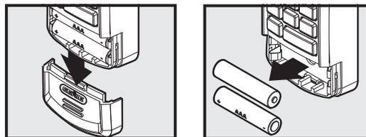
1. Remove battery cover and batteries.
