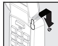
2. Drill 1/16" pilot hole for the top mounting screw (included).
