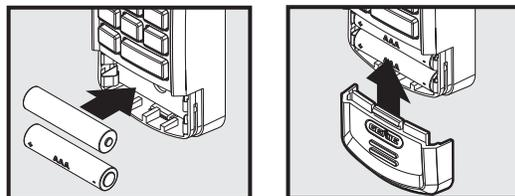
2. Replace batteries with same type batteries and check proper direction for (+) and (-) terminals.
