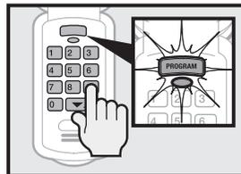
The Keypad's LED and Program key will flash slowly. Keypad lights will remain ON (for 30 seconds) if you have entered a valid PIN or have successfully programmed your Keypad.
