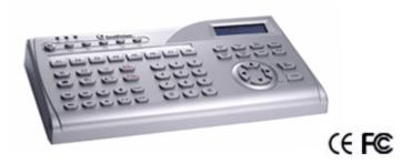
The GV-Keyboard V3 is used to program and operate GV-Systems and PTZ cameras. Through RS-485 configuration, it can control up to 16 GV-Systems. In addition, through RS-485 or RS-422 connection, it can set up and control up to 32 PTZ cameras directly without making anymogration through the GV-System.
