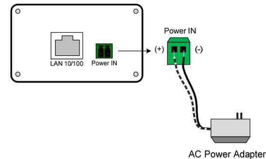
4. Connect the other end of the supplied **AC Power Adapter** to the power outlet. The Power LED on the front panel of the GV-PA191 turns green now.
