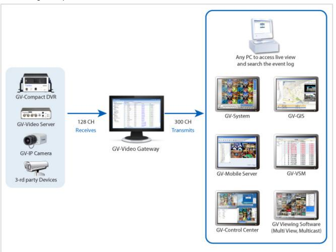
In some areas or countries, you may like to install 3G wireless Internet module (e.g. GPRS/UMTS) on the GV-Video Server or GV-Compact DVR but have the problem to obtain a public IP address from ISP. The Passive connection method of GV-Video Gateway can solve the public IP issue by accepting the connection request from the GV-Video Server or GV-Compact DVR, and then distribute the video streaming to clients.
