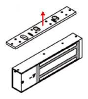
4. Attach the lock body to the L bracket and secure the mounting screws from step 2 using the inner hexagon wrench that comes with the GV-ML600.
