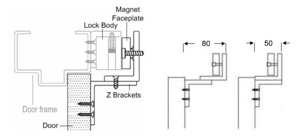
The L-Z brackets should look like the illustration below after installation is completed.
