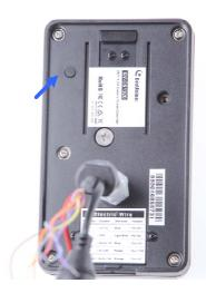
3. Wait until the status LED blinks twice to release the **Load default** button. The process takes about 5 seconds.
