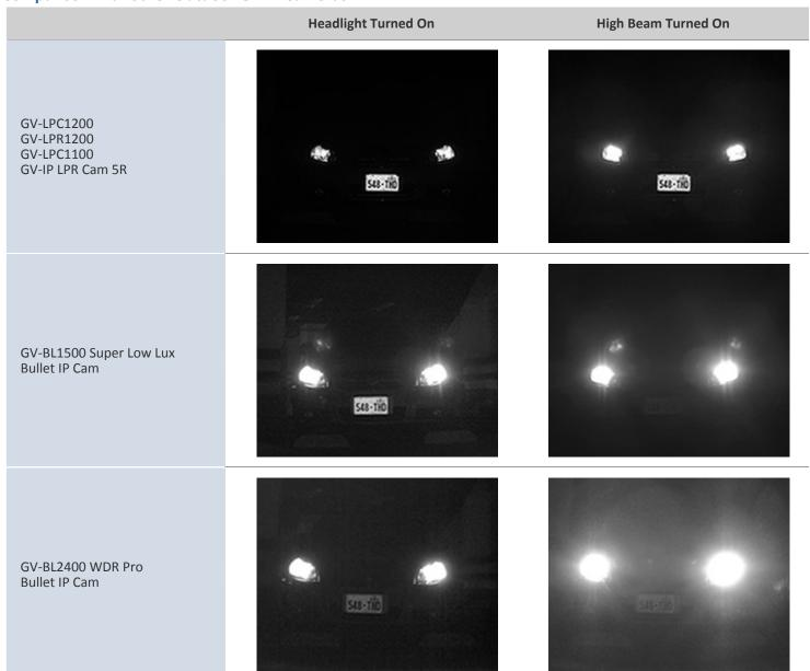
**Note:** The test results are based on the night scene. All cameras are installed at the distance of 10 m (32.81 ft) from the vehicle, with the resolution set as 1 MP or 1.3 MP and the shutter speed set as 1/2000 sec.
