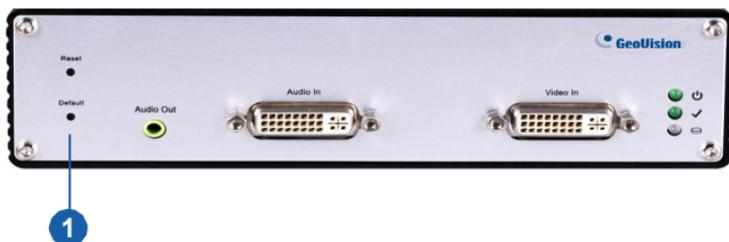
1. Press and hold the **Default** button until the Ready LED blinks. This may take up to 10 seconds. The Ready LED will blink twice.
