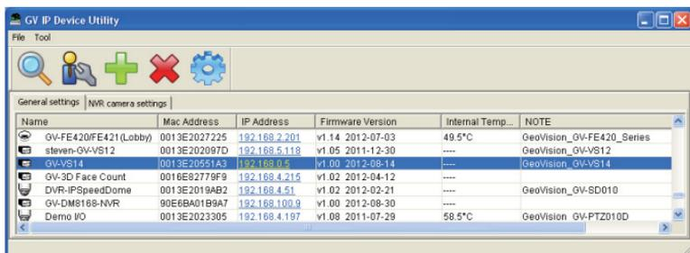
The screenshot shows the 'GV IP Device Utility' application window. It features a menu bar with 'File' and 'Tool', and a toolbar with icons for search, help, add, delete, and settings. Below the toolbar are two tabs: 'General settings' and 'NVR camera settings'. The main area contains a table with the following columns: Name, Mac Address, IP Address, Firmware Version, Internal Temp., and NOTE. The table lists several devices, with 'GV-VS14' selected.
