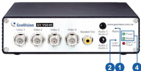
1. Press and then release the **Reset** button immediately.
